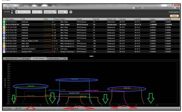
As the picture shows in this example, there are a number of different Wi-Fi networks in this particular surrounding. The signal strength varies in between them as shown with the blue markings. You can also see the channels used by those networks as shown with the red arrows. What is of interest now is to try to check channel overlap and possibly better channels to use. As you can see there are gaps in the overall 2.4 GHz band as shown with green arrows. This could be better choices for channels.
