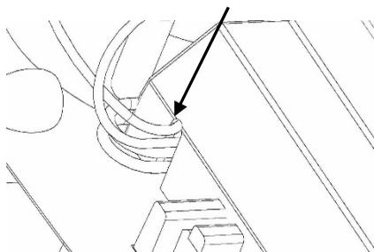
Pass the cable through the hatch and form a loop with the remaining cable, orienting it upwards before folding down the end of the cable and holding it in the clips, attaching the wires separately to the appropriate terminals.
