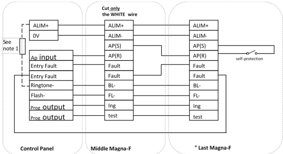
**Fig. 2 : Connection of MAGNA-F (multiple in waterfall)**
