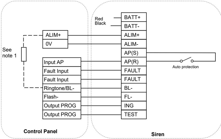
**Fig. 1: MAGNA-F connections (simple configuration)**
